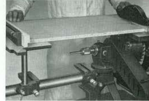
PANEL CUTTING using adjustable combination table. Capacity 9½" to 48". Note extension to fence of rebated timber to keep work steady.
