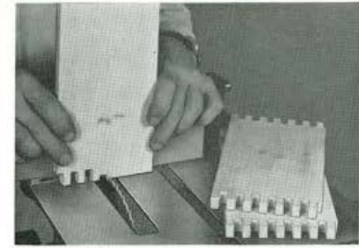
BOX COMBING. A 4" deep box accurately jointed in one minute. This operation normally takes hours by hand.
