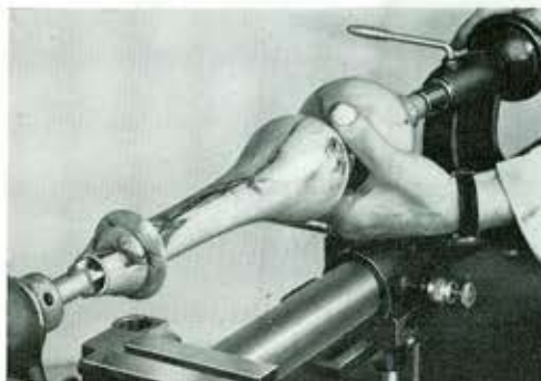
COUNTERBORE tool being used to bore for plug of capping.
