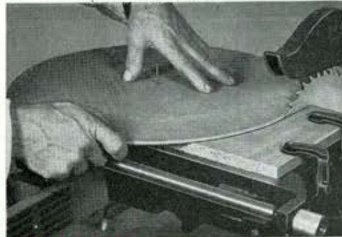
CIRCLE CUTTING using simple jig clamped to saw table. Workpiece pivots on nail, or use adjustable jig as illustrated on circular sanding.
