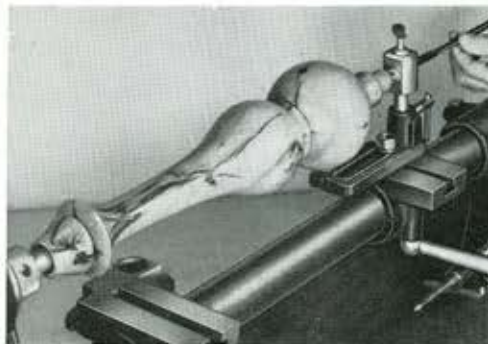
LONG HOLE BORING through body of chandelier, 5/16" dia. drill for standard electric fittings (Pillar Nipples)
