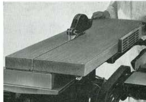
RIPSAWING with headstock swivelled to pass work along length of bed, utilising roller on rear of combination table fence. (Major Combination table only.)
