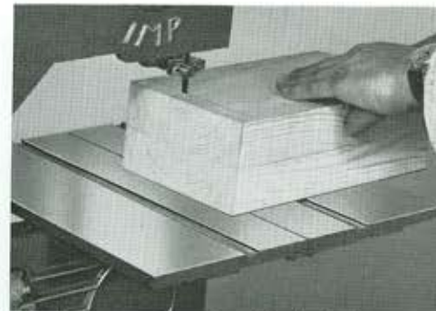
Using the deep cutting capacity of the Imp bandsaw to cross cut 7" x 4" timber. Feed rate 12" per minute.
