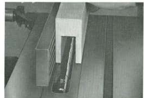
GROOVING, with Wobble Saw permits grooves of \frac{1}{4} " wide up to \frac{3}{4} " to be machined at one pass.
