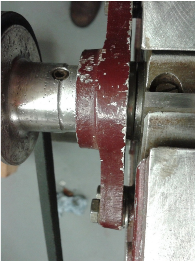
Plate 10 - Clearance between cutter block & bearing The two washers shown provide about 0.5mm clearance.
