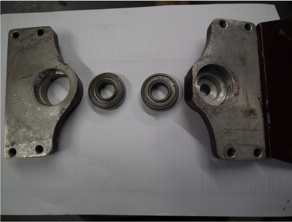
Plate 7 - Both inboard & outboard Bearing Housings with bearings removed
