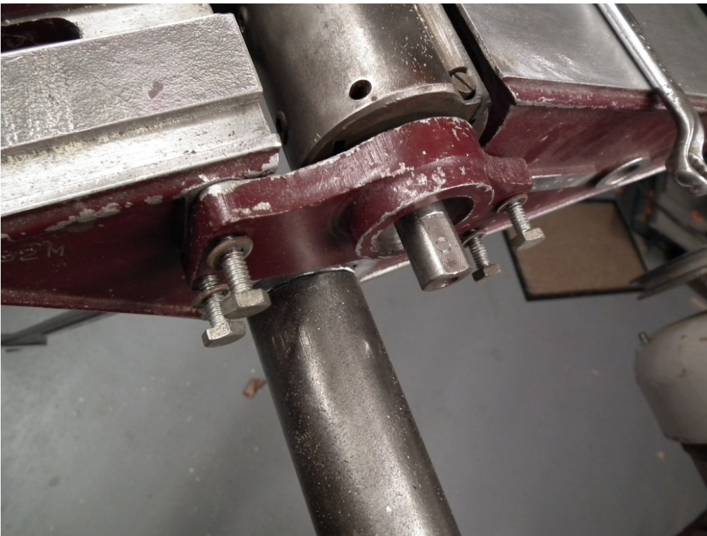
Plate 4 - Bearing Housing loosened (inboard)
