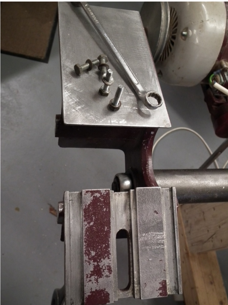
Plate 6 - The outboard Bearing Housing removed.
