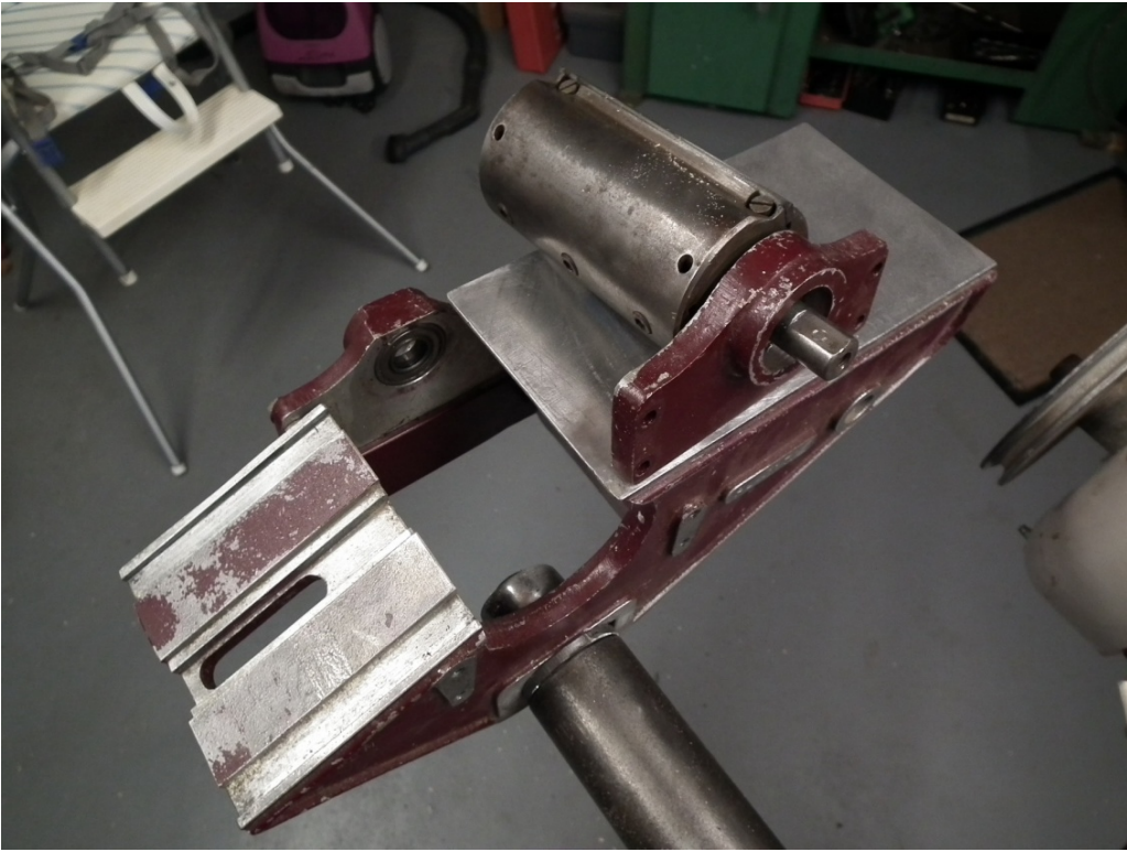
Plate 5 - Bearing Housing c/w cutting block removed. Note the inboard bearing housing still attached to the planer body.
