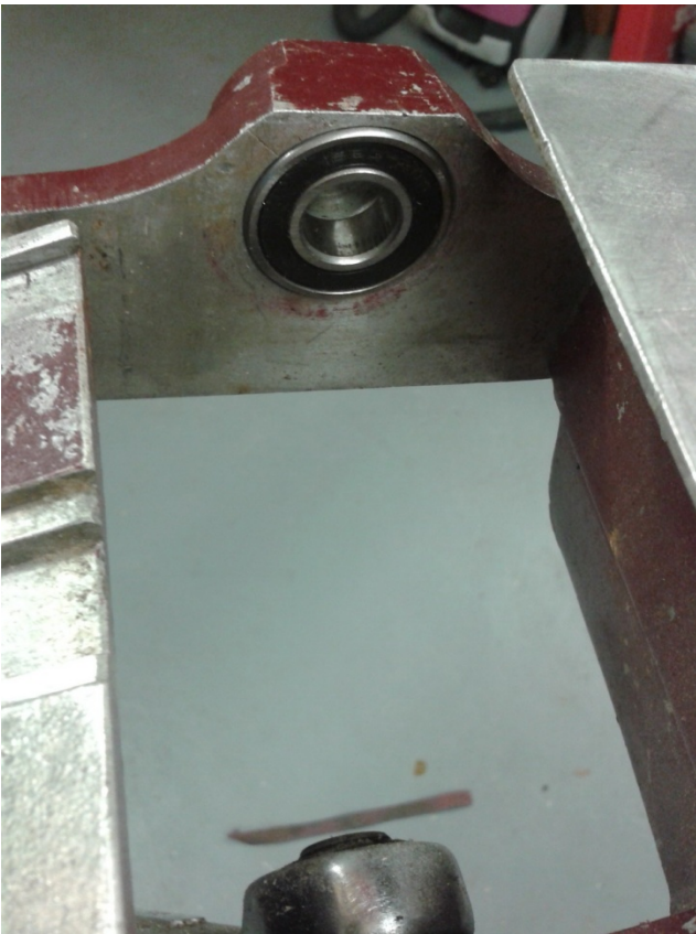
Plate 8 - New bearing in housing (outboard)
